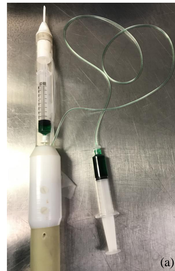
Figure 2: (a) A 10 cc syringe containing 1 mL of urease solution was placed in an animal bed and 3 cc of hyperpolarized sample was injected into the magnet with a connection line from out of the magnet, in order not to move the bed during the scan. (b) Conversion of HP ^{15}\text{N} Urea to \text{NH}_3/\text{NH}_4^+ . A ^{15}\text{N}/^1\text{H} 30 mm Doty coil was used to acquire spectra. (c) Conversion of HP ^{13}\text{C} Urea to \text{CO}_2/\text{HCO}_3^- . A ^{13}\text{C}/^1\text{H} 30 mm Doty coil was used to acquire spectra.
